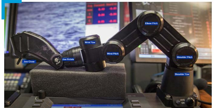
ROV pilots use this scale model to control D2's manipulator arm when collecting a sample. Image courtesy of Art Howard, GFOE; edited by Jeffery Laning, GFOE.
